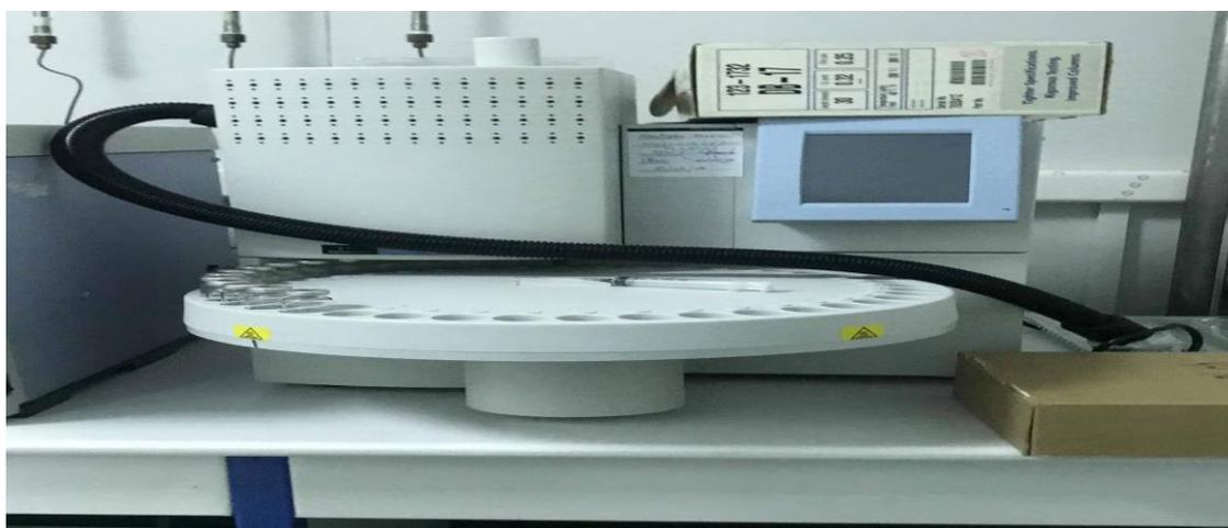
**Figure 28 :** Appareil CPG CLARUS 500 (Perkinelmer).
